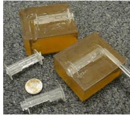
Fig. 19 Stereolithography mold pieces and camera roller prototypes
