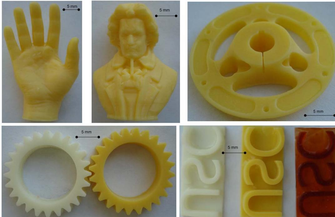
**Figure 13** Test cases for building objects in a single material
