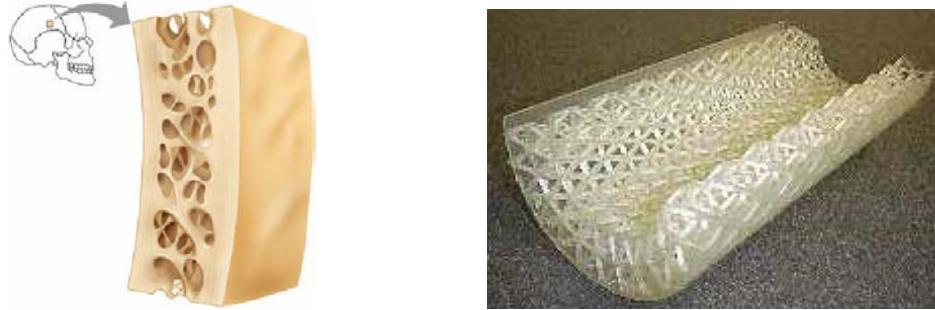
Fig. 2: Skull bones in human skeleton [5] (left) and a test part built by SLA [7] (right).
