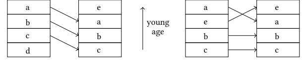
Figure 13: Update of the cache: two examples for a fully associative cache, with the LRU update policy.
