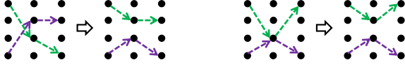
Figure 2: Two kinds of adjustment. Left: when two paths are crossing; Right: when two paths overlap.
