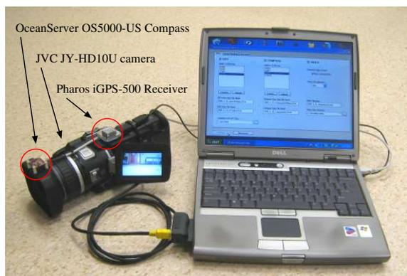
**Figure 1: Experimental hardware and software to acquire georeferenced video.**
