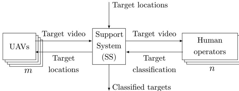
**Figure 2. Support System (SS) Architecture**
