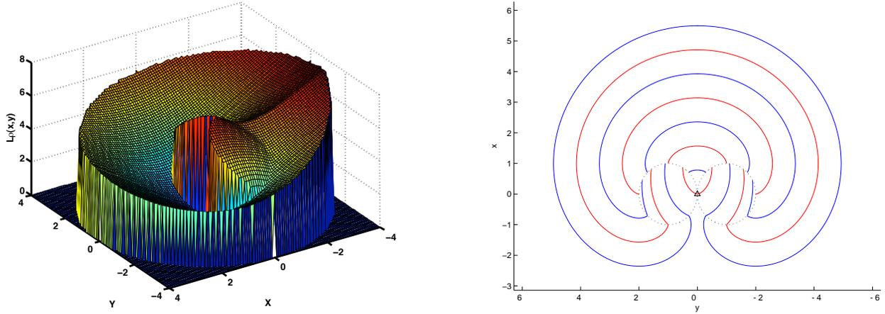
Figure 1. A 3D plot of the function  $L_\rho$  (left) and its level sets  $L_\rho$ , for  $\rho = 1$ , shown at increments of  $\pi/4$  (right). The initial vehicle configuration is represented by the black triangle, and is at coordinates  $(0,0)$  heading “up”. Note that the positive direction of the  $x$  axis is “up” and of the  $y$  axis is “left.”
