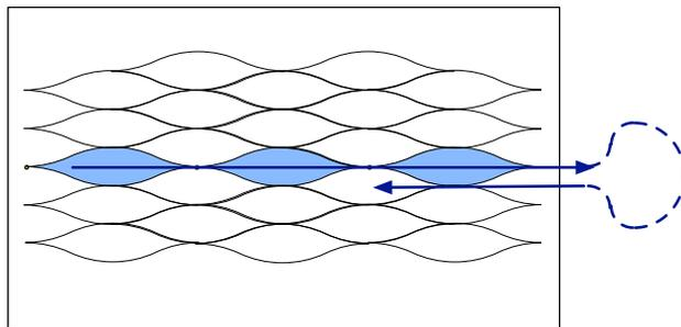
Figure 5. Sketch of the aligned periodic tiling and of the Bead-Tiling Algorithm
