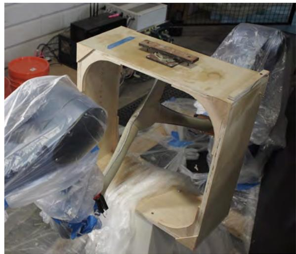
Figure 8: Fabric Forms Concrete casting with Kuka robots at UCLA Suprastudio
