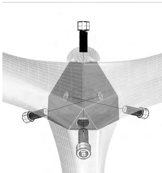
Figure 11: Fabric Forms Coupler bolting method
