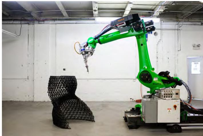
*Figure 5: 3D Printed Carbon Fiber-infused plastic from Branch Technology*
