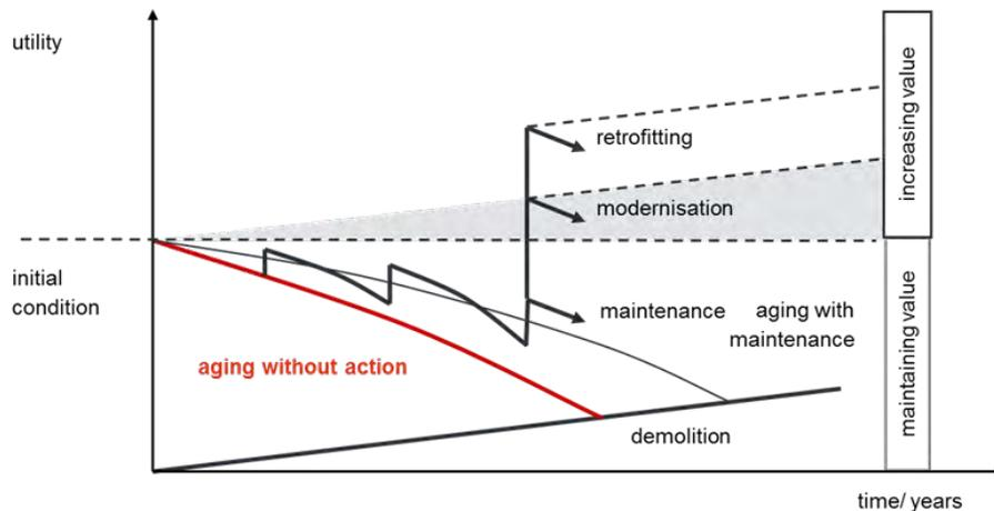
Figure.2: Options for extending the building life cycle, adding value and improving sustainability (Based upon Harfingier 2006) [2]
