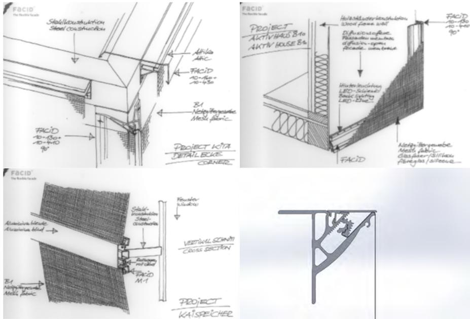
Figure 9: System profiles provide pre-designed solutions for most applications and form the basis for new façade ideas [6]
