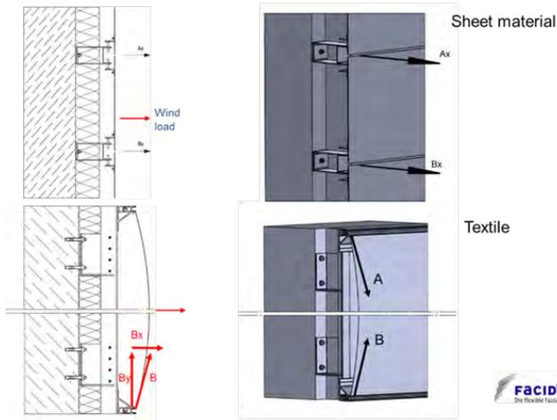
Membrane deflection and tension under wind load
