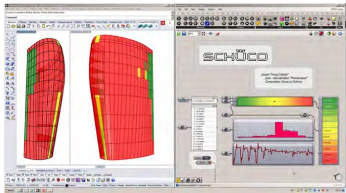
Figure 11: (Left): Example: Computational design tools used to plan and evaluate complex interactions between façade elements. (Right): Example: Grasshopper model. [7]
