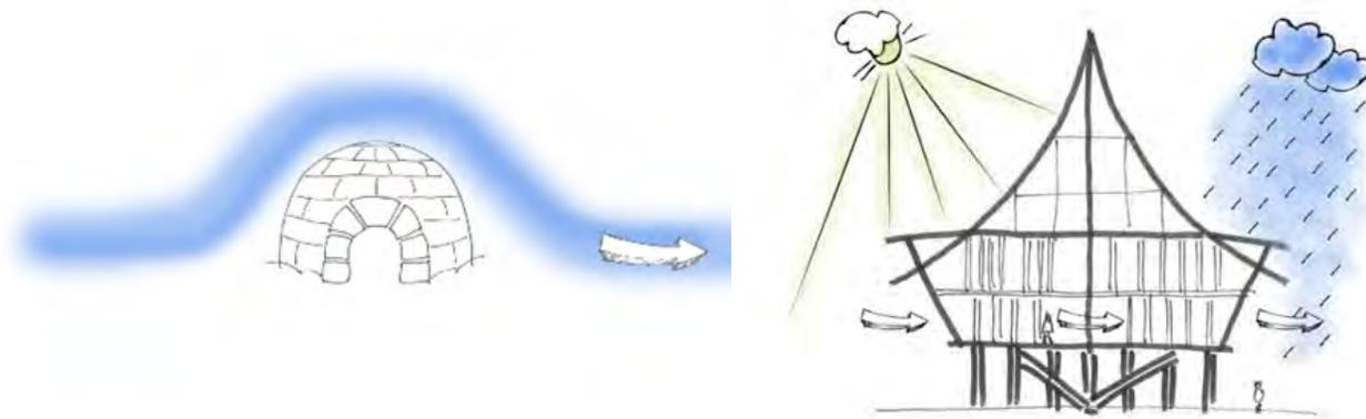
Figure.4: Examples of climatically inspired design; the arctic igloo (left) and (right) the tropical long house
