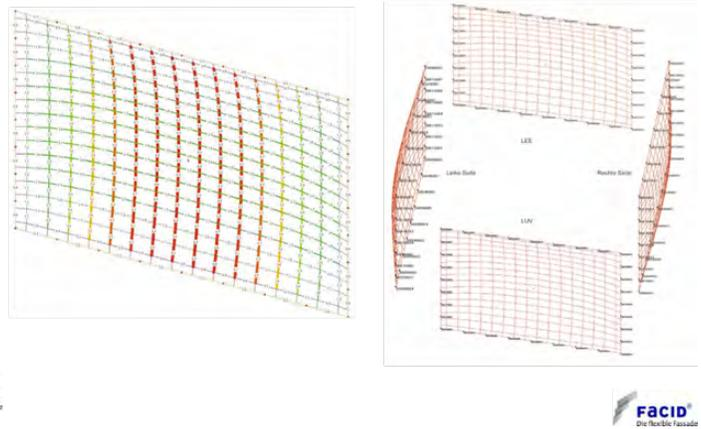
Figure 12: (Left) Structural requirements for frames tensioning textile coverings are more challenging than for solid sheet materials. (Right): Structural analysis of the textile skin enables the correct frame profiles for the tensioning load to be chosen. [6]
